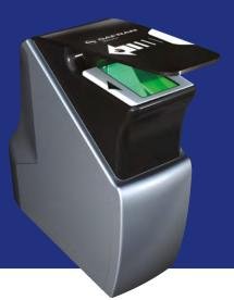
MorphoWave<sup>™</sup> is a contactless fingerprint acquisition solution. This innovative device captures four finger images with a single movement in less than a second. Its dynamic acquisition capability allows subjects to be 'on the move' during fingerprint capture. MorphoWave<sup>™</sup> is well suited for high traffic environments.
