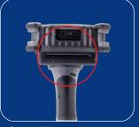
Contact/Contactless smartcard reader for credential verification.
