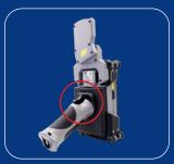
Handgrip with trigger for convenient barcode scanning.
