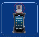
HID NOMAD FAP 30 fingerprint reader on swivel mechanism that can be stowed when not in use.
